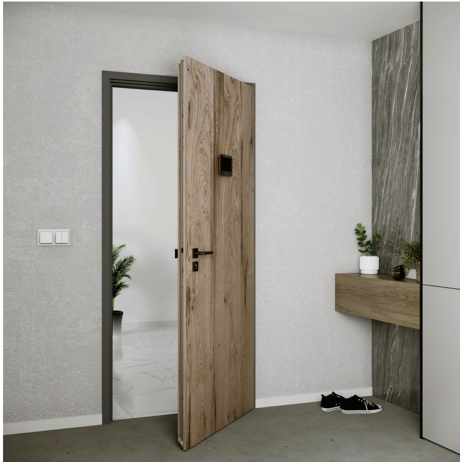
interior view: ELEGANT 10 - beam oak veneer, Super White oil / SAP 871 doorframe in RAL 7024, fire resistance 30 min., security class RC3, acoustic rating 43 dB, climate III, M9 security hardware, Eques S1 Pro digital door viewer
