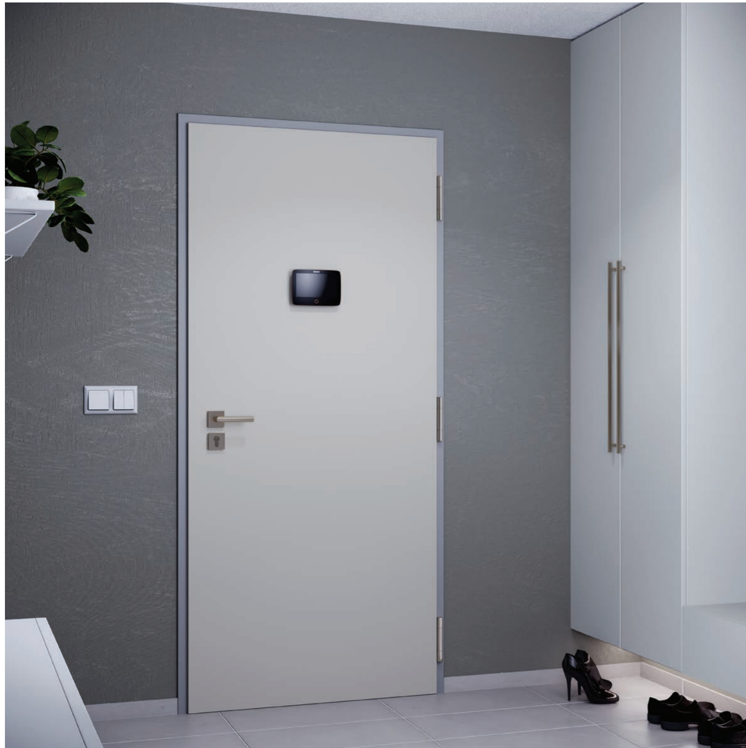
interior view: ELEGANT 10 - HPL Antifinger light grey U708 / SAP 865 metal doorframe in RAL 7035, fire resistance 45 min., security class RC3, acoustic rating 37 dB, climate III, M9 security hardware, Eques S1 Pro digital door viewer
